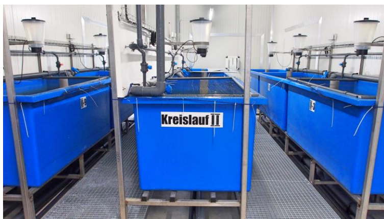
Figure 1. Recirculating aquaculture system (RAS) operated in the NEMATIC pilot facility at the FishGlassHouse (FGH), University of Rostock. The system consists of nine culture tanks (left) and a water treatment unit (right) including a sedimentation tank for mechanical filtration and a trickling filter for biological treatment.
