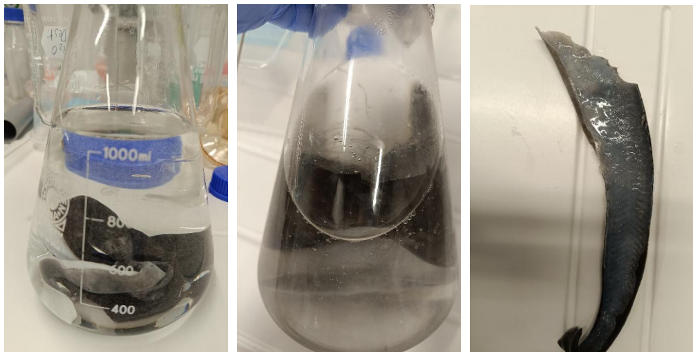
Figure 7: Just after the skin was placed in the NaOH; after 24h in NaOH, mucus and other tissues are dissolved in the solution; skin weight is now 44.8 g.
