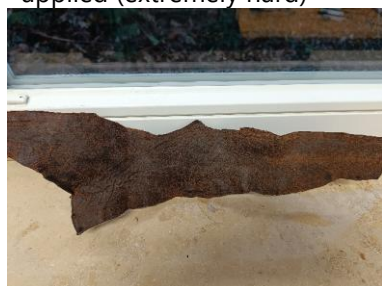
Figure 16: a) African catfish skin 1 days in the tannin solution, b) Olive and coconut oil were applied (softer but still room for improvement)
