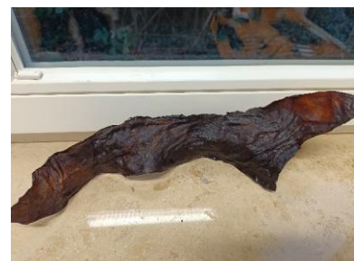
Figure 15: a) African catfish skin 3 days in the tannin solution, b) only coconut oil was applied (extremely hard)
