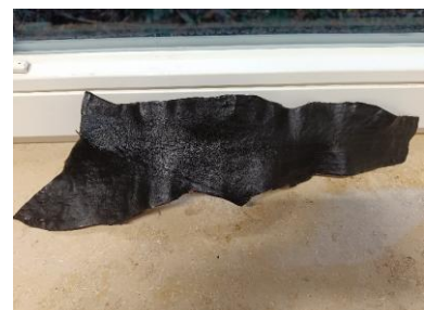
Figure 16: a) African catfish skin 1 days in the tannin solution, b) Olive and coconut oil were applied (softer but still room for improvement)
