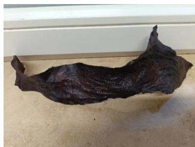
Figure 15: a) African catfish skin 3 days in the tannin solution, b) only coconut oil was applied (extremely hard)
