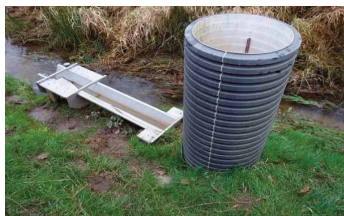
Fig. 4 A filter device as an end-of-pipe solution for the removal of phosphorus from tile drainage water. The filter barrel is equipped with iron-coated sand, which has been found suitable for phosphorus adsorption and which is a by-product of the drinking water industry
